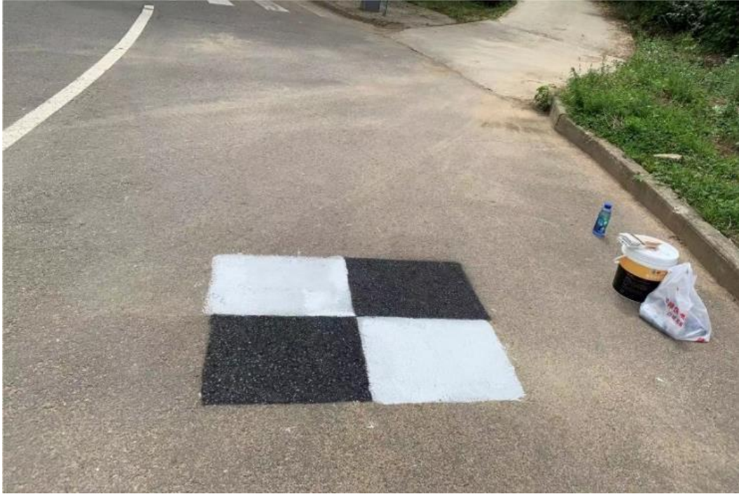
Figure: Example of a 3D checkpoint in the field (the white paint is highly reflective while the black paint is non-reflective)
