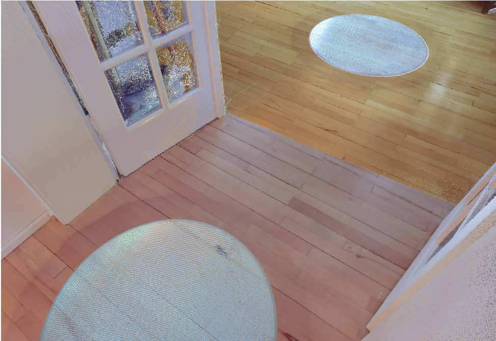
Figure 10-61 Inconsistent color of a floor due to scans taken under varying lighting conditions.
