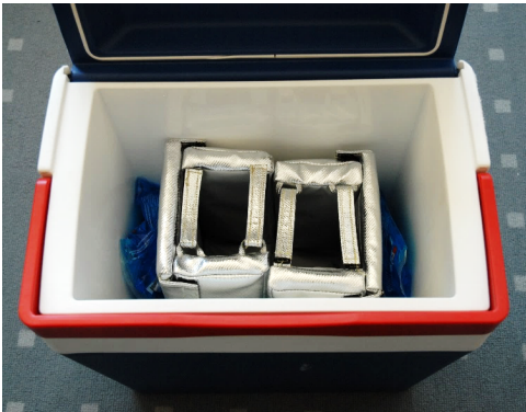
Figure 3-2 : Set of pre-cooled thermal insulation covers inside an insulated cooler
