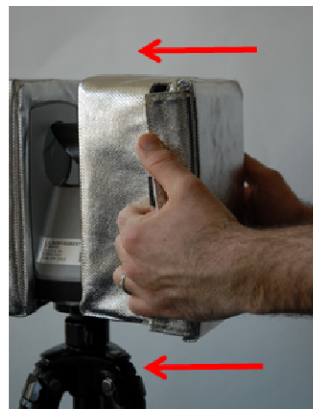
Figure 3-5 : Slide thermal protection cover onto scanner
