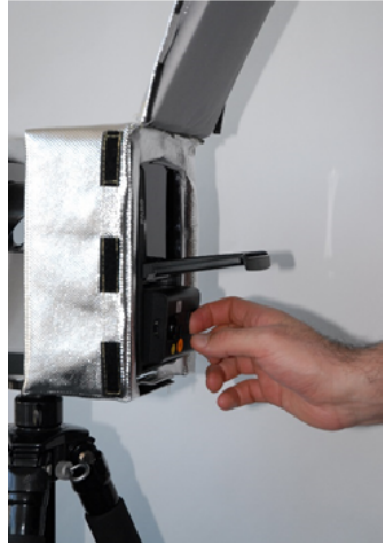
Figure 3-10 : Access to Power Pack and Battery
