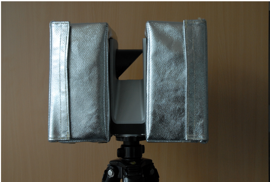
Figure 3-1 : FARO thermal protection covers
