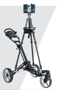
As its name implies, Swift is fast – capable of capturing large and complex areas in as little as 10 minutes. While already the most accurate mobile 3D laser scanning system for large areas, Swift is also capable of taking stationary scans with unmatched detail.
